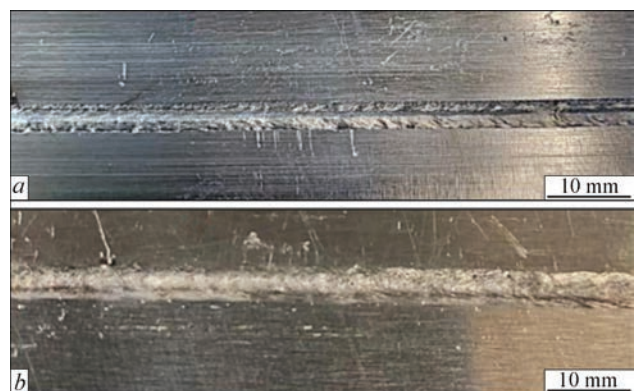
Figure 5. Appearance of welded joints of alloys 5251 with 6082 [30] (thickness 1.5 mm) in the TWB (tailored welded blanks) products produced by electron beam (a) and laser (b) methods
