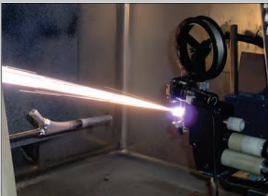
Deposition of coatings from titanium wire by microplasma spraying
