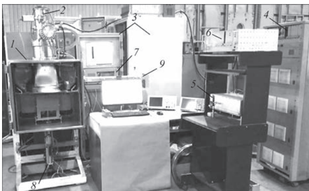
Figure 3. Equipment for electron beam 3D-printing (designation 1–9 see in the text)
