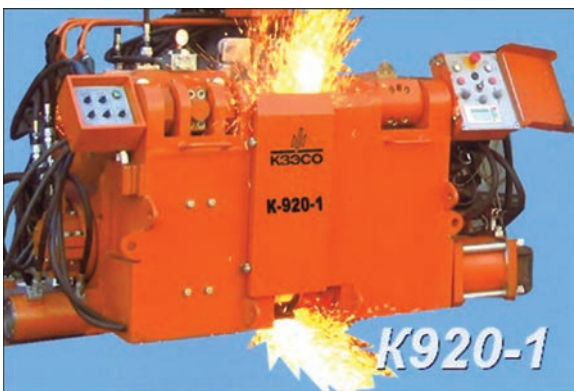
Figure 2. Rail welding head K920-1
