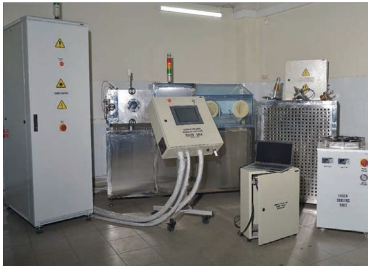
Figure 9. Complex for laser, microplasma and laser-microplasma welding in a controlled atmosphere and in a dynamic vacuum
