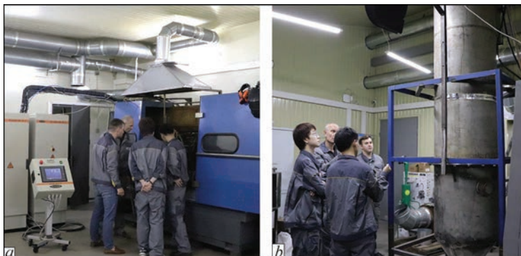
Figure 11. Equipment for realization of plasma-arc technologies for spraying of coatings and treatment of materials: a — universal technological complex of plasma-arc spraying and cutting; b — experimental installation for plasma-arc spheroidization of wire materials and rods and powders of irregular shape
