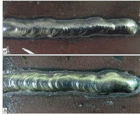
Figure 5. Surfaced samples produced with twin electrodes with independent power supply (for description of a , b see the text)
