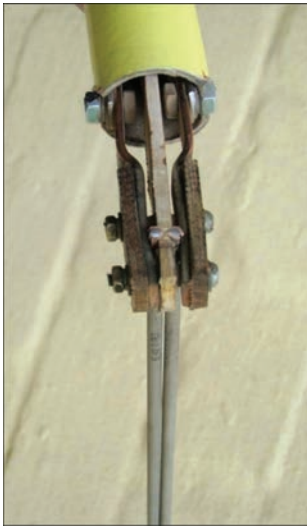
Figure 4. Photo of electrode holder with independent power source
