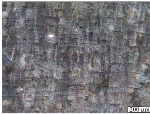
Figure 5. Structure of experimental specimen No. 6 (initial state after manufacturing)
