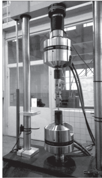
Figure 2. MTS318.25 testing complex with fixed Zr-coated samples
