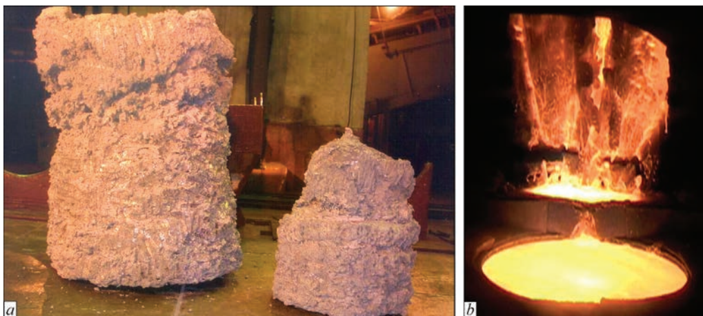
Figure 3. EBM of sponge titanium blocks; a — 4 t sponge titanium block, compared to 0.7 ton block; b — EBM of 1100 mm dia. ingot from uncrushed sponge titanium blocks
