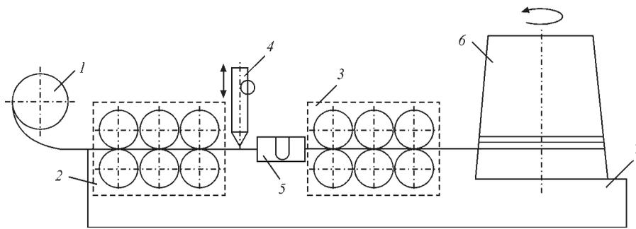
**Figure 1.** Schematic of a drawing machine for producing titanium flux-cored wire: 1 — cassette; 2, 3 — roller stands; 4 — dosing unit; 5 — U-shaped strap; 6 — drum; 7 — page
