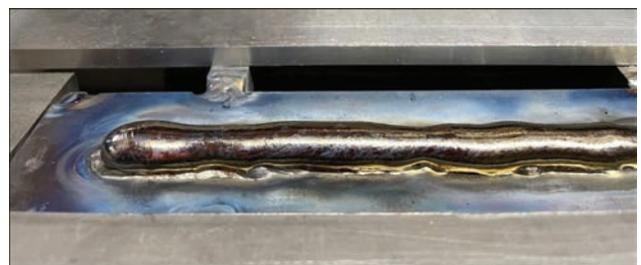
**Figure 7.** General view of a five-layer sample after the process of deposition with flux-cored filler wire based on T120 titanium alloy
