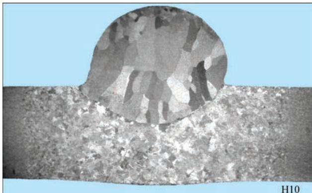
**Figure 4.** Macrosection of the produced three-layer sample made with flux-cored filler wire based on titanium alloy VT22
