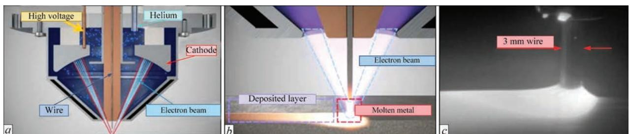
**Figure 9.** Configuration of xBeam® 3D Metal Printing process: xGun design schematic (a); configuration of a heated zone in the feed point during deposition (b); photo of the actual deposition process (c) [21]
