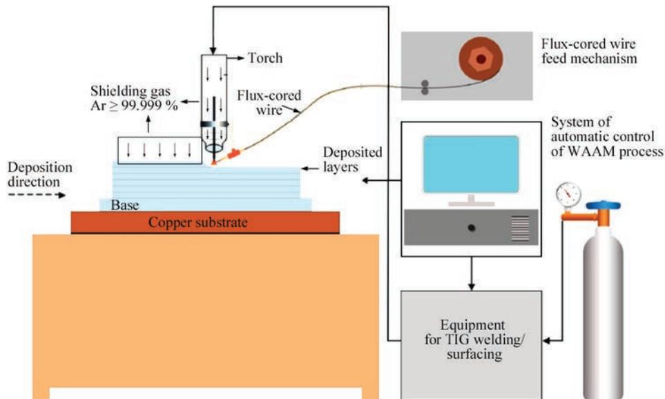
**Figure 3.** Schematic of a unit for layer-by-layer TIG deposition using metal-cored filler wire
