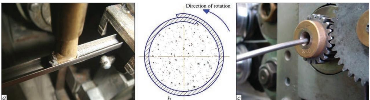
**Figure 2.** Process of forming and further pulling of metal-cored wire: *a* — charge dosing; *b* — sheath closing scheme; *c* — rotating die
