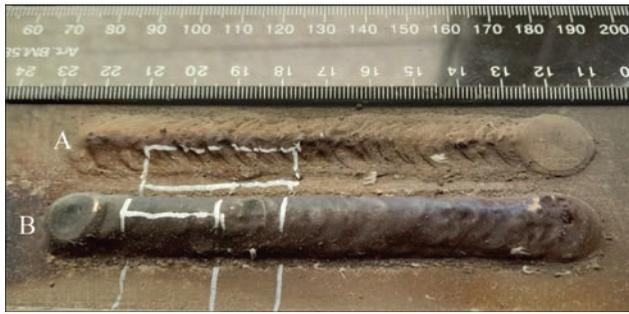
**Figure 10.** General view of the samples: A — single-layer; B — multilayer
