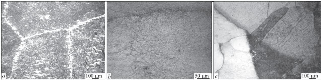
**Figure 6.** Microstructure of a three-layer sample made with application of flux-cored filler wire based on VT22 titanium alloy: *a* — base metal; *b* — weld metal; *c* — fusion zone
