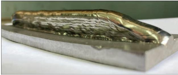
**Figure 8.** General view of a nine-layer sample after the process of deposition with metal-cored filler wire based on Ti alloy of Ti-Zr-Nb system
