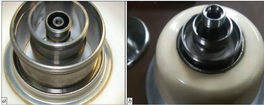
Figure 6. General outside (a) and inside (b) appearance of repaired CU of EBG
