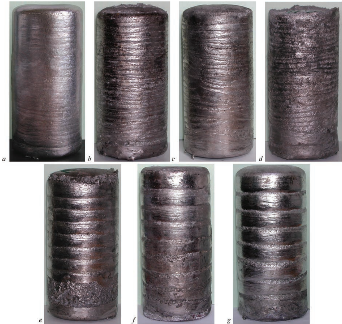
Figure 3. Appearance of titanium ingots, melted by ESR with the use of a longitudinal pulsed magnetic field: a — B = 0.24 T, t_{\text{pulse}} = 0.3 s, t_{\text{pause}} = 10 s; b — B = 0.24 T, t_{\text{pulse}} = 1.0 s, t_{\text{pause}} = 10 s; c — B = 0.24 T, t_{\text{pulse}} = 1.5 s, t_{\text{pause}} = 10 s; d — B = 0.24 T, t_{\text{pulse}} = 2.0 s, t_{\text{pause}} = 10 s; e — B = 0.22 T, t_{\text{pulse}} = 11 s, t_{\text{pause}} = 21 s; f — B = 0.16 T, t_{\text{pulse}} = 11 s, t_{\text{pause}} = 33 s; g — B = 0.16 T, t_{\text{pulse}} = 21 s, t_{\text{pause}} = 33 s
