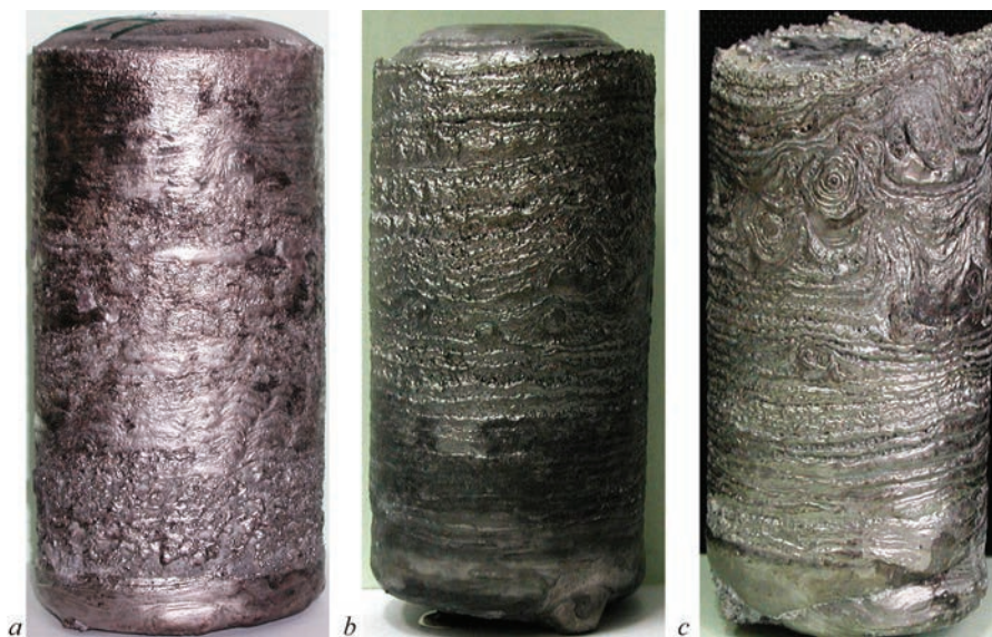
Figure 2. Appearance of titanium ingots, melted by ESR using a longitudinal permanent magnetic field of a different induction, T: a — 0.16; b — 0.24; c — 0.30
