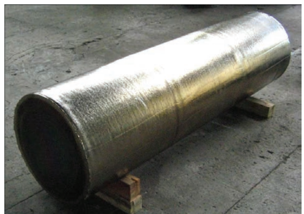
Figure 5. Ingot of high-temperature titanium alloy VT9 of 600 mm diameter with a surface-melted side surface
