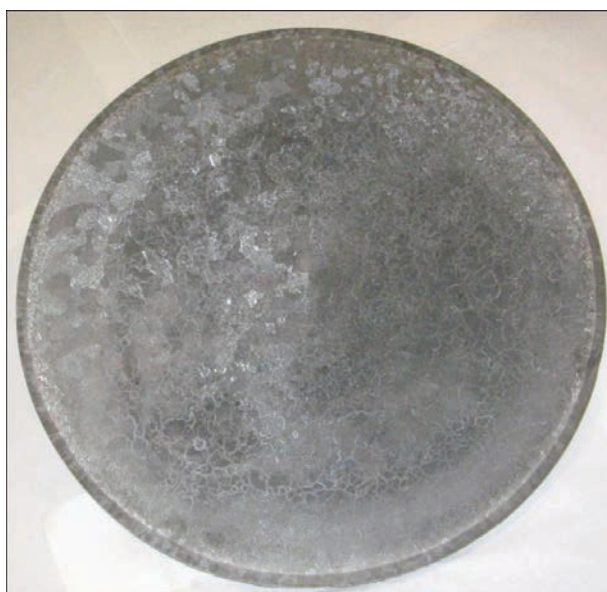
Figure 6. Macrostructure of metal of ingot of high-temperature titanium alloy VT9 of 600 mm diameter with a surface-melted side surface
