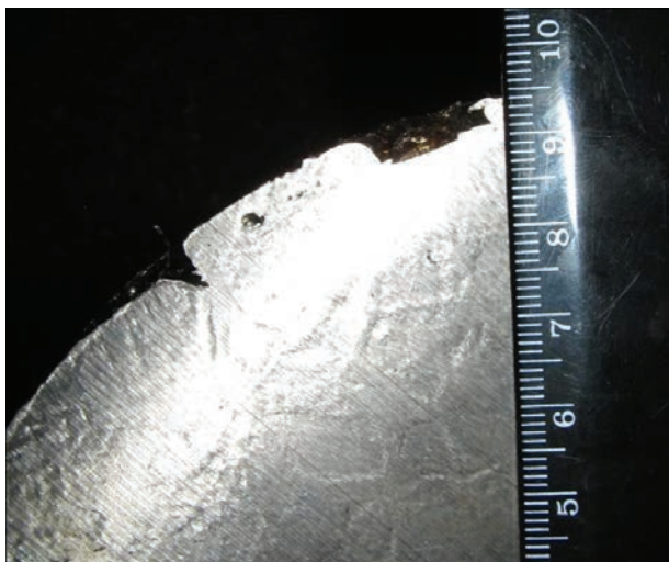
Figure 10. Defective layer of ingot surface
