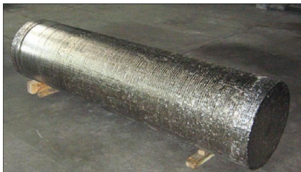
Figure 1. Ingot of high-temperature titanium alloy VT9 with a diameter of 600 mm, produced by EBM method
