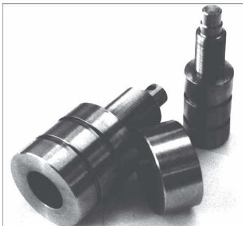
Figure 6. Parts of electroslag titanium after mechanical cutting treatment, \times 0.5
