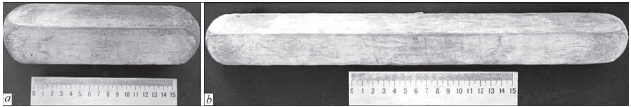
Figure 8. Appearance of deformed titanium semi-finished products with varying degrees of deformation, %: a — 45; b — 90
