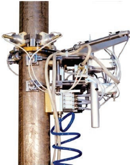
Figure 3. EC scanner of CRAB system installed on pipe of secondary reforming furnace
