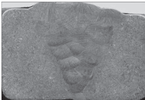
Figure 4. Macrosection of CA-6NM steel welded joint
