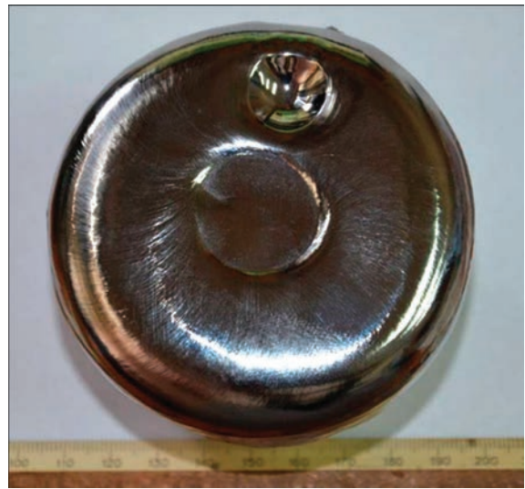
Figure 5. Outer surface of the embryonic crystal before the experiments on growing the walls of the hollow single-crystalline cylinder
