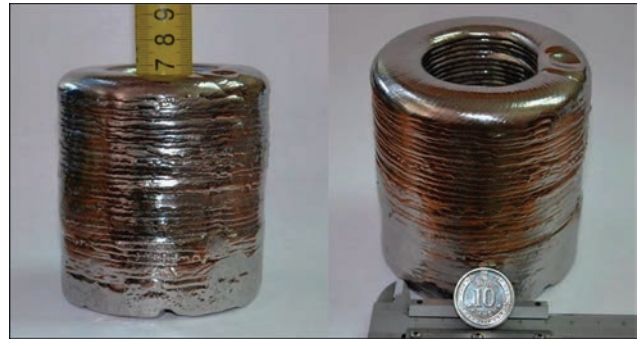
Figure 8. Appearance of tungsten single-crystal in the form of a hollow body of revolution of 85 mm diameter
