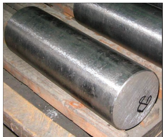
Figure 9. Machined ingot of Ti-6Al-7Nb titanium alloy
