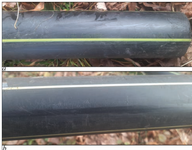
Figure 2. Specimens of polyethylene pipes from PE-80: ST1 (a) and ST2 (b)
