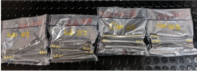
Figure 4. Specimens of vacuum packed polyethylene pipes for structural studies
