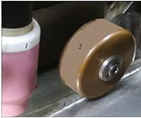
Figure 1. Process of 3D printing with plastic deformation of the deposited layer by electrodynamic treatment: 1 — torch for 3D printing; 2 — cylindrical electrode-indenter with the contact surface in the form of a straight line; 3 — printed layer of metal
