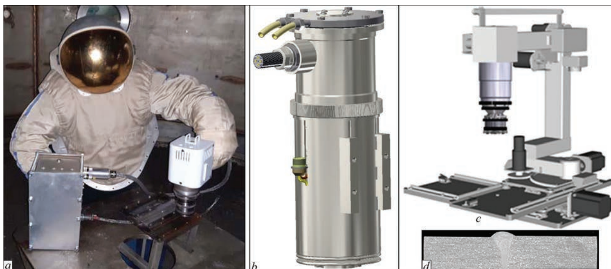
Figure 8. New generation manual electron beam tool and gun for welding and 3D printing for long-term operation: a — prototype of hand tool complex tested during performance of technological experiments; b — general view of electron beam gun for welding in space as part of a manipulator or robot; c — special 5-axes manipulator developed for performance of automatic welding; macrostructure of 8 mm AMg6 aluminium alloy
