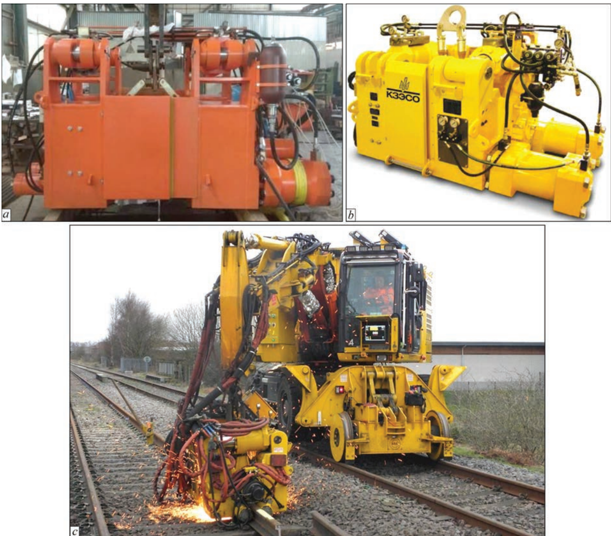
Figure 12. Mobile machines K960 (a), K945 (b), rail welding complex with K945 machine (c) for FBW of rails with “tension”
