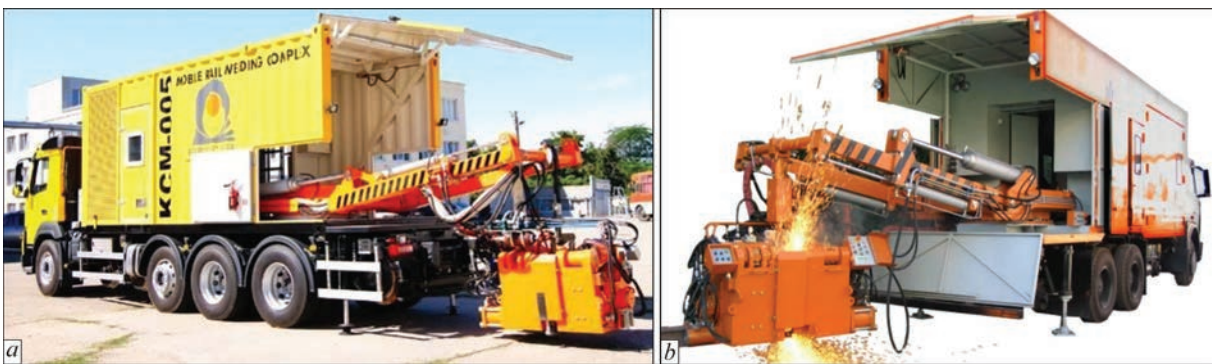
Figure 14. Rail welding complex KCM 005 on a combined chassis equipped with machine K920 (a), K922-1 (b)
