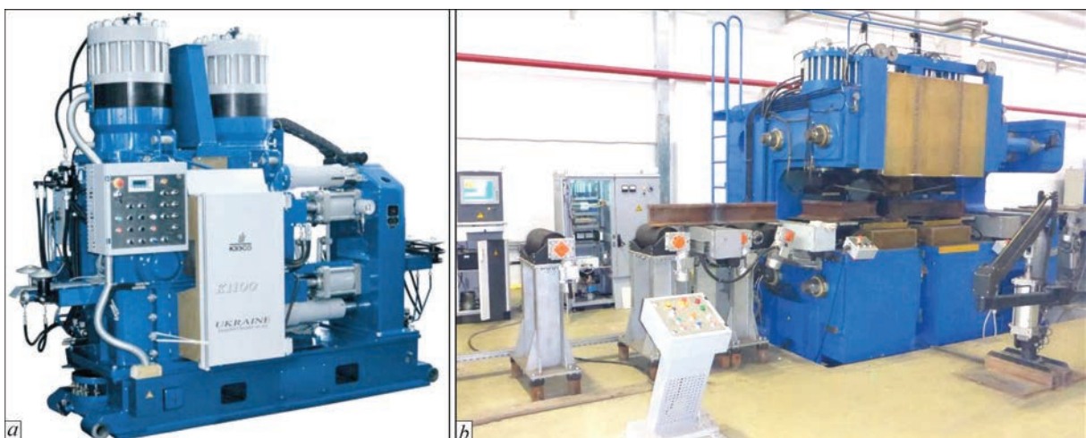
Figure 10. Stationary rail welding units K1100 (a), K924 (b) designed at PWI
