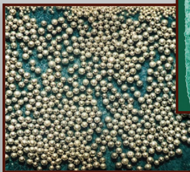
Appearance of spherical tungsten carbides
