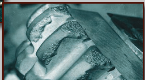
Characteristic wear of drill bit teeth clad with tungsten carbide
