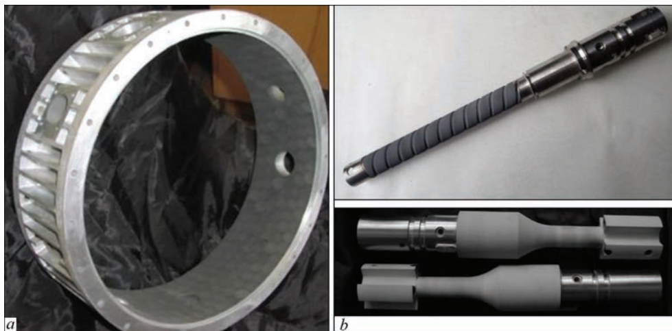
Figure 9. Light alloy parts: a — rotary piston engine housing; b — drill telemetry parts
