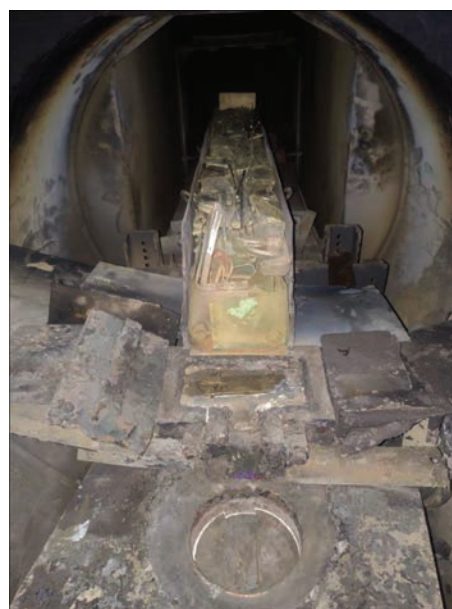
Figure 2. Initial charge from low-grade nickel scrap
