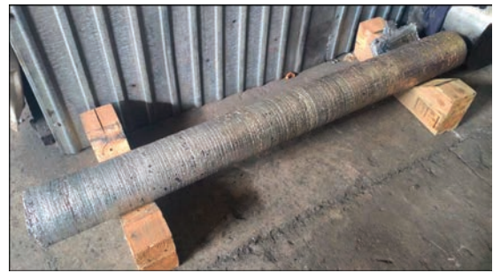
Figure 4. EBR nickel ingot of 150 mm diameter
