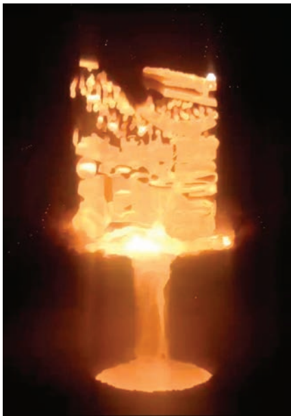
Figure 3. Process of electron beam remelting of nickel
