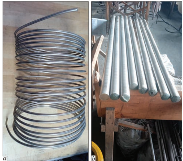
Figure 5. Semi-finished products from EBM nickel of NP2 grade: a — 3 mm wire; b — drawn soft rods of 40 mm diameter
