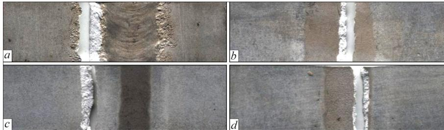
Figure 5. Appearance of the face (*a, c*) and root (*b, d*) surfaces of the working part of GTA welded specimens of 2 mm MA2-1M magnesium alloy with weld reinforcement (*a, b*) and without it (*c, d*)
