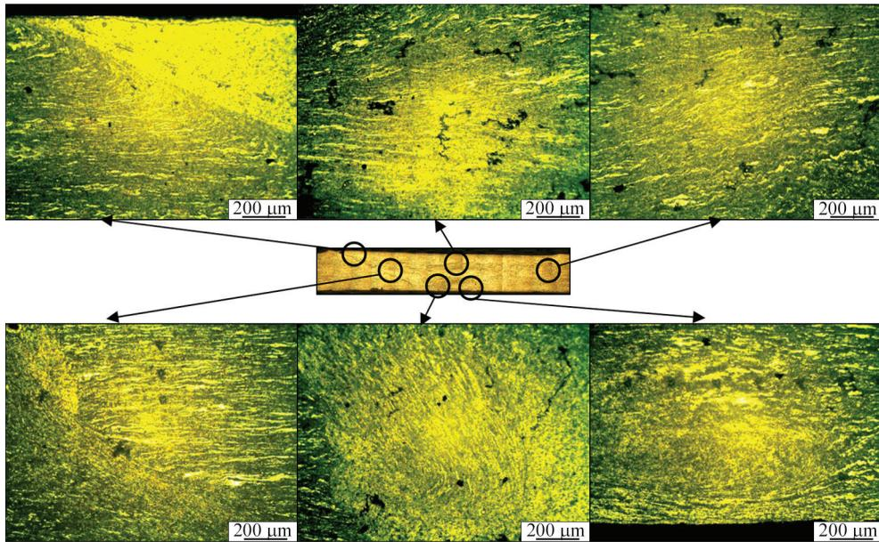
**Figure 1.** Fragments of the microstructure of FSW butt joint of structural MA2-1M magnesium alloy
