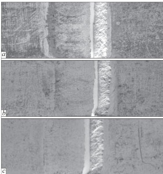
**Figure 3.** Appearance of the face surface of working part of 2 mm MA2-1M magnesium alloy specimens fractured as a result of static tension, which were produced by FSW at welding speeds of 8 (a), 16 (b) and 24 m/h (c)
