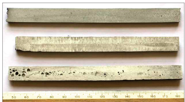
Figure 6. Macrostructure of the longitudinal section of rods with different nitrogen content, %: 1 — 0.73; 2 — 0.74; 3 — 0.9
