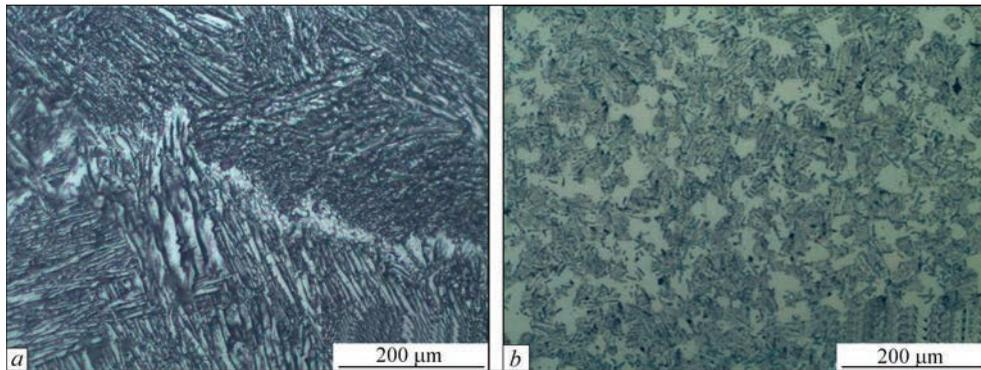
**Figure 9.** Microstructure of ingots after etching: *a* — without modifiers; *b* — with modifiers,  $\times 200$
