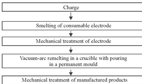
**Figure 1.** Scheme of the technological process for manufacturing titanium aluminide products
