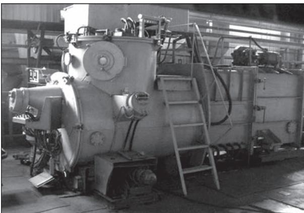
**Figure 2.** Appearance of electron beam unit UE-208M
