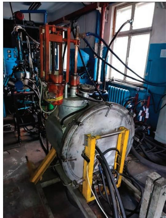
**Figure 4.** Arc furnace with nonconsumable electrode
