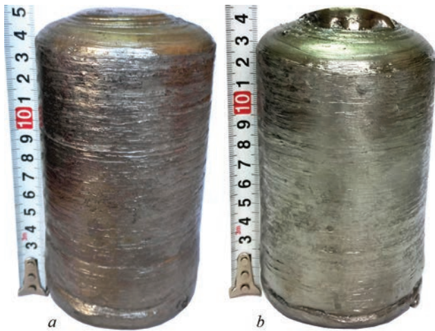
Figure 2. VT1-0 titanium ingots melted at a pressure of 25 kPa (a) and 160 kPa (b)
