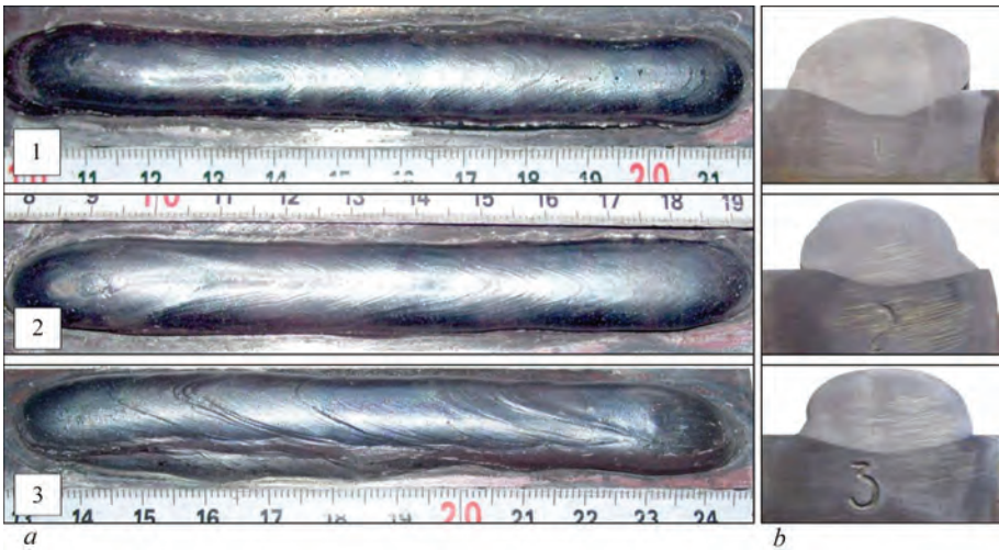
Figure 1. Appearance of samples deposited with wires Nos 1–3 in five layers (a), and their transverse macrosections (b)
