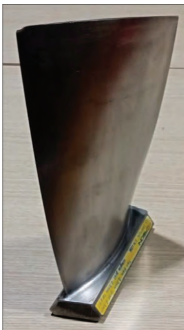
Figure 1. Typical gas turbine compressor blade with an electro-erosion slot of 4 mm long, 0.2 mm deep and opening of 0.1 mm in the fillet zone for adjustment and checking of the inspection technique
