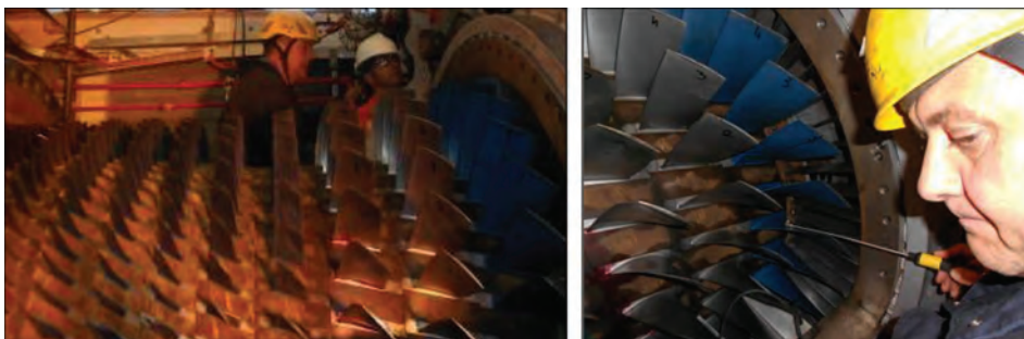
Figure 9. In-service tests of the proposed eddy-current inspection technique of gas turbine blades
