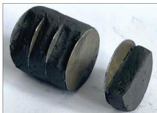
Figure 10. Raw sandwich made from preceramic precursor paste obtained from zirconium oxide–ammonium paratungstenate–cobalt acetate tetrahydrate–amorphous boron–sucrose system
