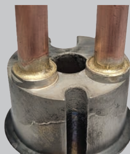
Brazed gas discharge gun assemblies for melting, coating and additive manufacturing
