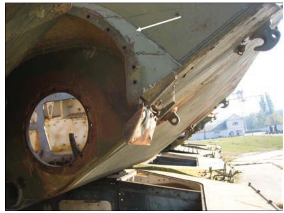
Figure 1. Fatigue crack in a welded joint of a LAV product after long-term operation
