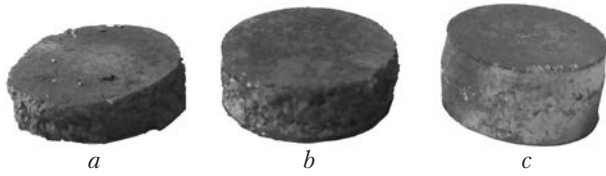
Fig. 2. The view of the samples after testing the raw pressing strength: a – mixing; b – mechanosynthesis; c – copperizing
