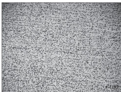
Fig. 7. The structure of the base metal
