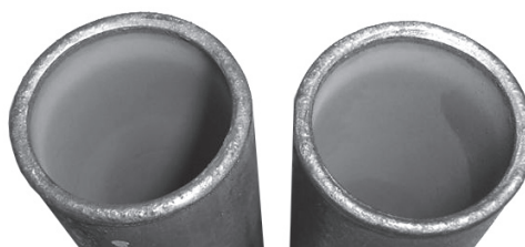
Fig. 9. Appearance of the pipe butts before upset
