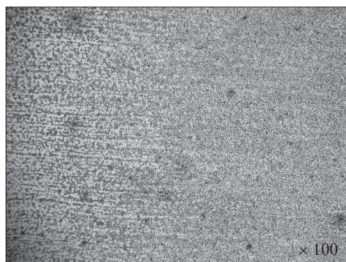
Fig. 6. Complete recrystallization area of HAZ
