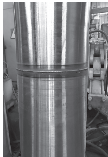
Fig. 3. Welded pipe joint, diameter of 212 × 3 mm
