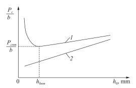
*Fig.* **1**. Qualitative dependences  $P_c/b = \varphi(h_0)$  during cold rolling, calculated with taking into account (curve 1) and without taking into account (curve 2) the influence of elastic deformations of rolls and strip
