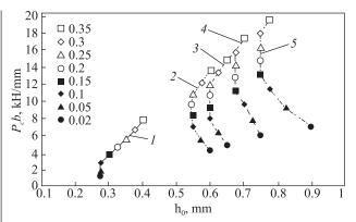
**Fig. 3.** Dependences  $P_{\text{cHA}}/b = \varphi(h_{0\text{HA}})$ , constructed from the results of modeling the parameters of cold rolling of 08kp steel strips (R = 300 mm, f = 0.05;  $q_0 = q_1 = 0$ ) with different degrees of preliminary work hardening:  $1 - \varepsilon_{\text{np}} = 0$ ;  $2 - \varepsilon_{\text{np}} = 0.4$ ; 3 - the same 0.5; 4 - the same 0.7; 5 - the same 0.9
