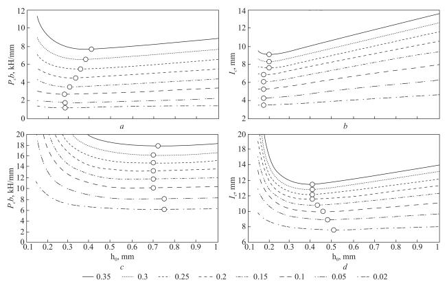
*Fig. 2.* Dependences  $P_c/b = \varphi(h_0)$  and  $l_c = \varphi(h_0)$ , constructed from the results of modeling the parameters of cold rolling of non-riveted ( $\varepsilon_{np} = 0$ ) (*a*, *b*) and work-hardened ( $\varepsilon_{np} = 0.75$ ) (*c*, *d*) strips made of 08kp steel (R = 300 mm, *f* = 0.05; q\_0 = q\_1 = 0)
