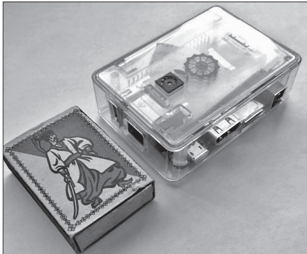
Fig. 2. Special video camera based on Orange Pi Lite microcomputer and OV5640 sensor
