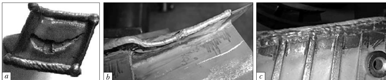
Fig. 8. Studied modern GTE part samples, used to research effect of process gas quality and content effect on nickel-based super alloy MPWD process: a – D-18T GTE HPT blade, ZhS32-VI super alloy; b – HPT nozzle vanes sector, ZhS6K super alloy; c – jet nozzle sash, VH4L super alloy
