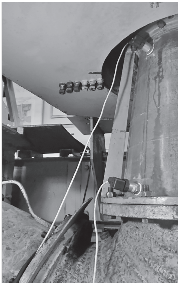
Fig. 4. Placement of sensors on the draft tube diffuser
