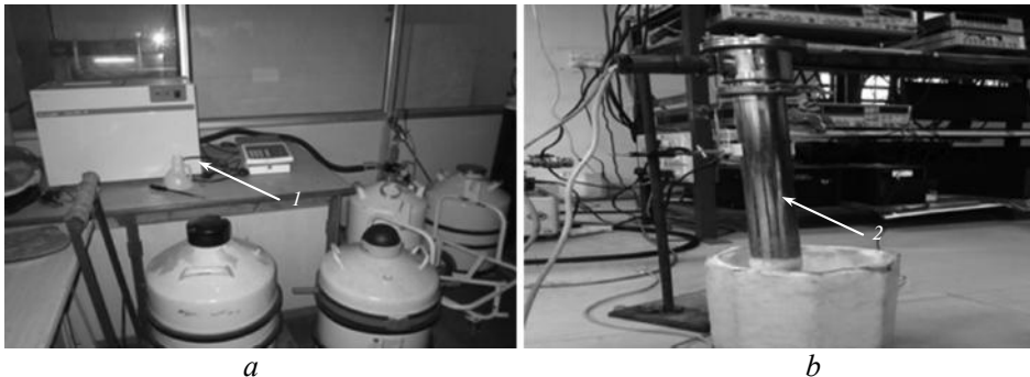
Fig. 1. Experimental setup for shallow cryogenic treatment ( a ), and deep cryogenic treatment ( b ): 1 – cryo chamber; 2 – dipstick.
