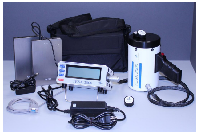
Fig. 4. Portable electronic emissometer/reflectometer TESA 2000
