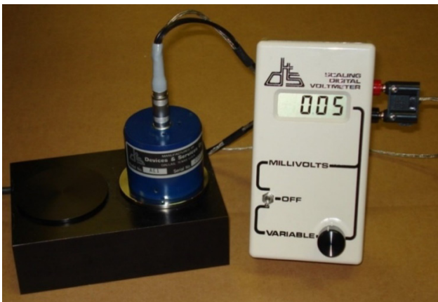
Fig. 3. Emissometer model AE1 of the firm Devices & Services Co. (D&S) [27]
