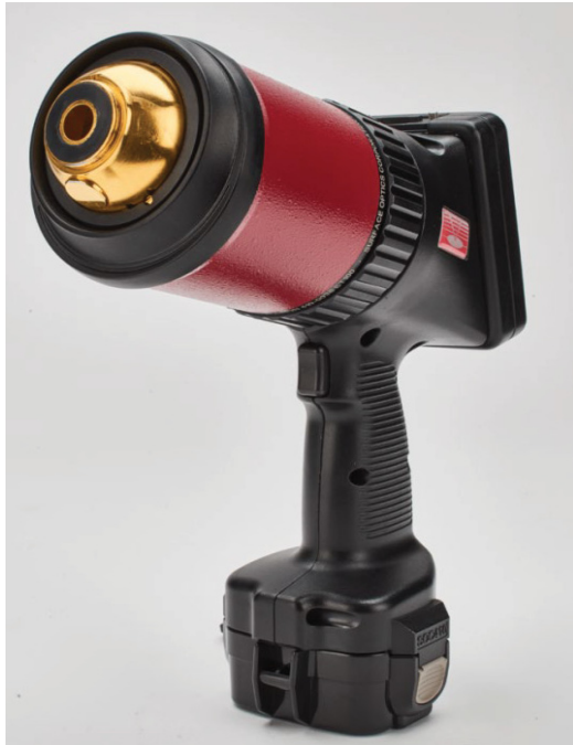
Fig. 5. Manual emissometer/reflectometer ET-100 [29]
