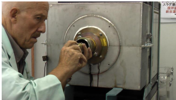
Fig. 5. Mounting of the light-guide thermometry system on heating furnace (Nippon Steel and Sumitomo Metal Corporation – Japan, Kimitsu, 14.07.2011)
