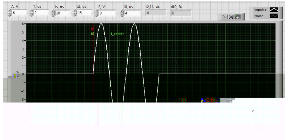
Figure 7. Determination of the onset of pulse in the case of low pulse polarity
