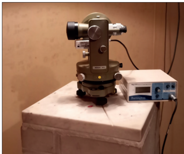
Figure 1. Non-magnetic theodolite Wild T1 with fluxgate MagA and magnetometer Mag-01H
