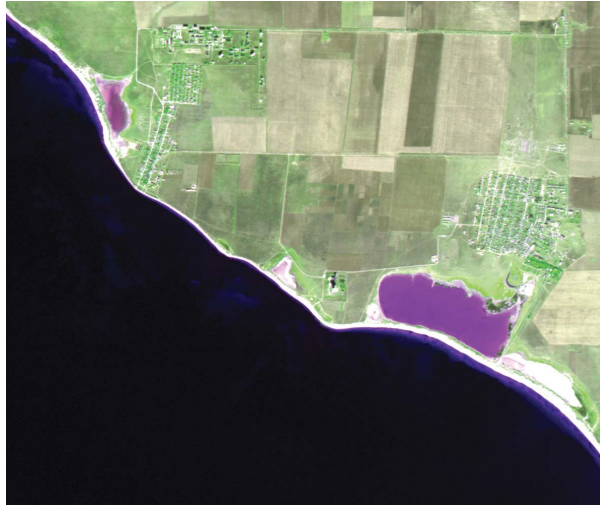
Fig. 1. “Sich-2” multispectral satellite image NSFCTC, November 8, 2011, 7.8 m spatial resolution, spectral bands 2 (0.61-0.68 \mu\text{m} ), 3 (0.79-0.89 \mu\text{m} ), 1 (0.50-0.59 \mu\text{m} )
