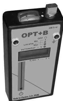
Photo 2. Portable track finder with voltmeter ORT+V.
