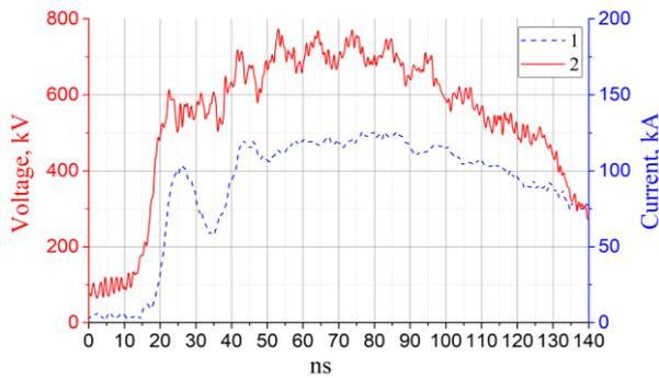
Fig. 3. Voltage and current waveforms. 1 – current (Rogowski coil); 2 – voltage (resistive voltage divider). (See color Figure on the journal website.)
