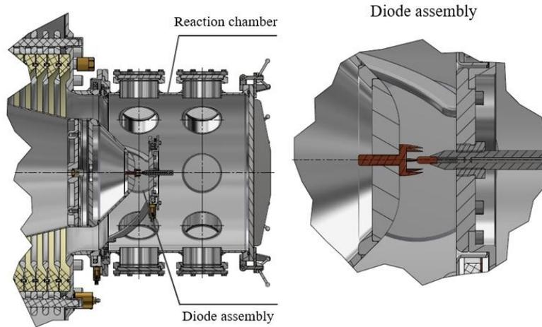
Fig. 2. Sketch of the reaction chamber and diode of the “ShAD”. (See color Figure on the journal website.)
