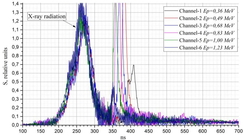
Fig. 7. Oscillogram of signals from scintillation detectors in the Thomson mass analyzer within the basic position  $M/Z = 1$  (experiment SH42881). (See color Figure on the journal website.)
