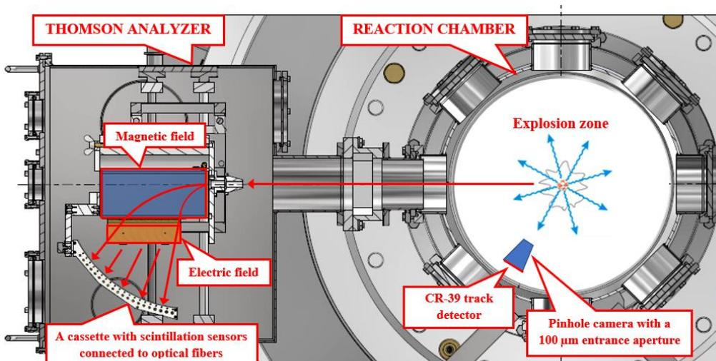
Fig. 5. Schematic view of the reaction chamber of the ShAD unit and diagnostic tools. (See color Figure on the journal website.)
