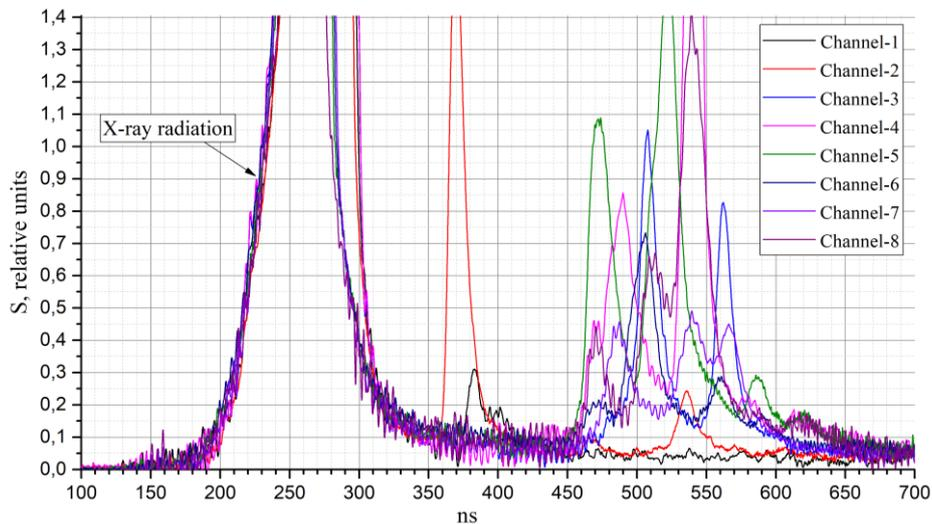
Fig. 8. Oscillogram of signals from scintillation detectors in a Thomson mass analyzer with the electric field turned off (experiment SH42918). Channel-1 –  $E_p = 0.36$  MeV; channel-2 –  $E_p = 0.49$  MeV. (See color Figure on the journal website.)
