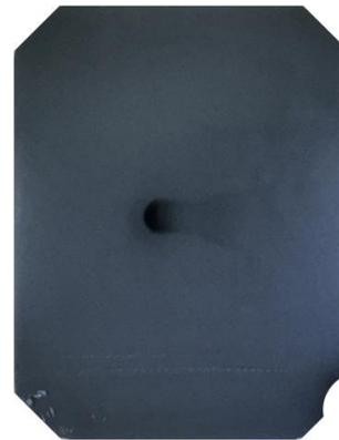
Fig. 4. Image of a 6.0 mm target anode in X-rays, using SD-Speedx film, class D, size 30 × 40 (experiment SH42944).
