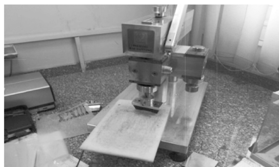
Figure 3 Dumbbell shape cutter instrument according to ISO-527
