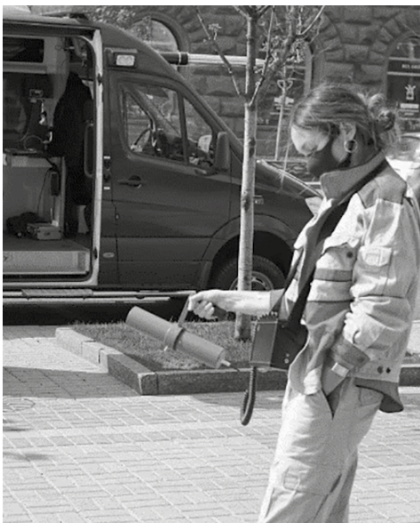
Figure 2 – SSTC NRS emergency crew performing radiological survey in Kyiv after a storm during wildfires in the Chornobyl Exclusion Zone (April 2020)
